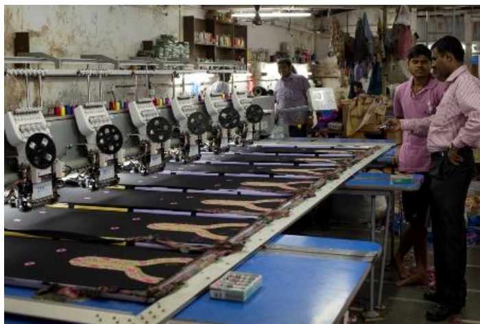
Picture 1 – Multi – head machine in an embroidery unit in Mumbai
